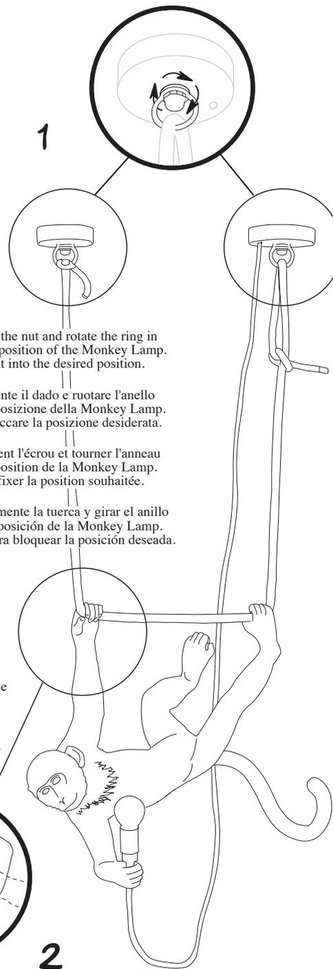
Slightly unscrew the nut and rotate the ring in order to adjust the position of the Monkey Lamp.
